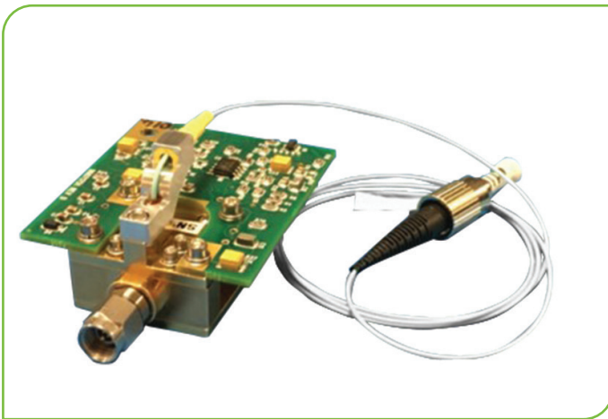
Custom-designed OEM OE Converter installed into sampling oscilloscope
